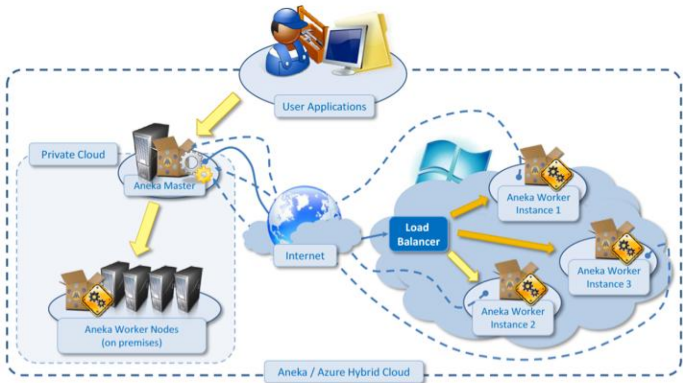
Figure 6: Schematic of Aneka/Azure Interaction for data analytics application [45].
